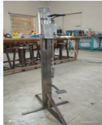
Mechanical pedal fixed hand free dispenser for hands sanitization by KAHE
